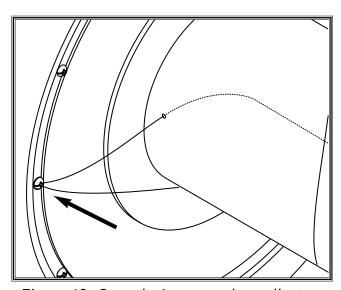
Figure 19. Ground wire secured to collector.
